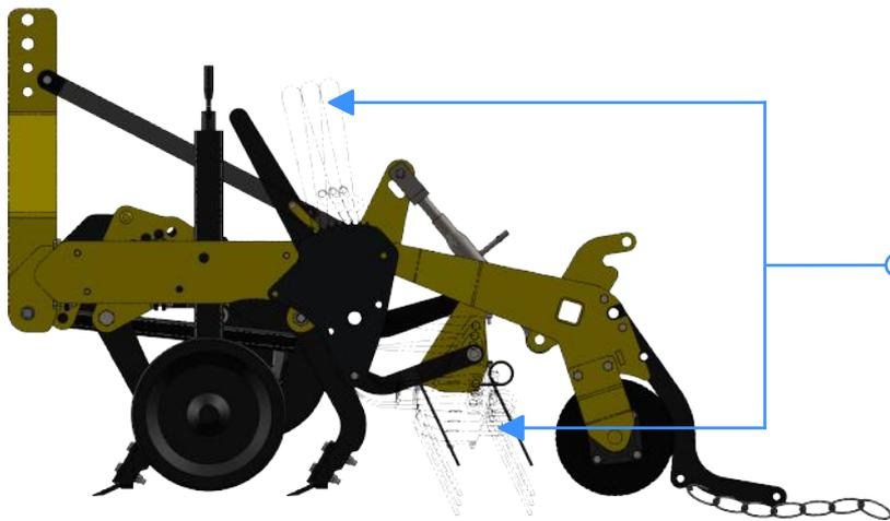
LA POSITION DES HERSES EST FACILEMENT RÉGLABLE PAR UN SEUL LEVIER. ELLE RESTE FLOTTANTE EN PERMANENCE POUR SUIVRE LE PROFIL DU SOL.
